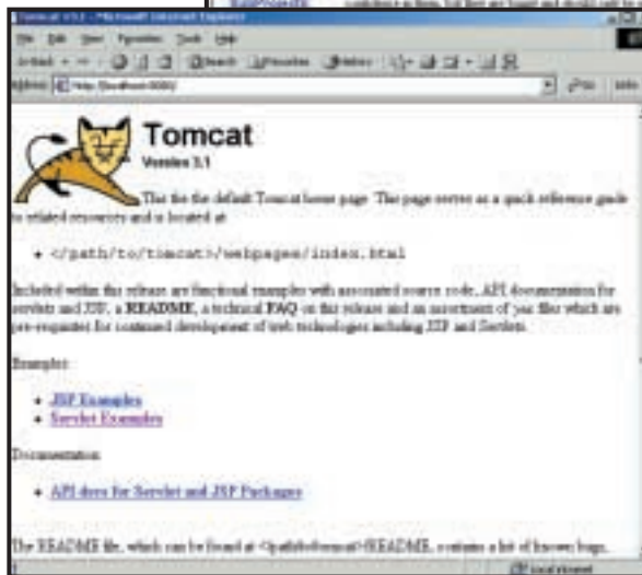
If you get this web page, your local Tomcat installation has been successful
